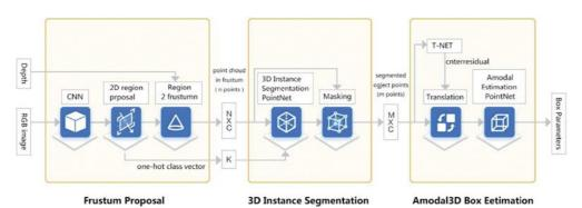
Exclusive Design of LiDAR Holographic Point Clouds Algorithms Architecture
